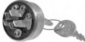
SSW2817 Key Switch Lawn & Garden Applications PIC 9900-9017; 3-Position 5-Terminal 5/8 Mounting Stem Can Use SSW9200 Wiring Harness Used on Honda H1011, H1011H, H1011HK1, H2013SA, H2013SAC, H2013HK1SAC John Deere JD321 Commercial Walk Behind Mowers, 111 Series (Below 1200) Toro Sand Pro Aerators, Greensmaster 3000G, and Reelmaster 216 REPL.: AYP / ROPER
