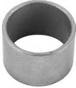
SMT7121 Bushing, C/S For Mitsubishi Starters PIC 6-16016; ID 14.1mm; OD 16.1mm; OAL 10.9mm; Used on Mitsubishi OSGR Starters
