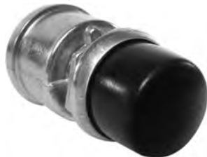
SSW2814 Push Button Switch PIC 9900-9014; 2-Screw Terminals ON-OFF (Normally OFF) Switch 2 Threaded Bosses with Screws for Wire Connections Plastic Button O-Ring Seal in Mounting Stem Protective Cap and Face Nut Assembly REPL.: COLE HERSEE 90030-01, 90030BP, 9095, 9244, 9244-02, 9245; DELCO D907
