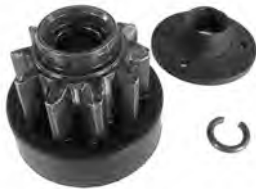
STC5312 Drive Assy. CCW; 10-Tooth; For Tecumseh Starters PIC 6106-6404; Gear OD 32mm Gear ID 10.2mm OAL 32.6mm Includes Nut on Back of Drive Lester 5747, 5754; REPL.: TECUMSEH 36853
