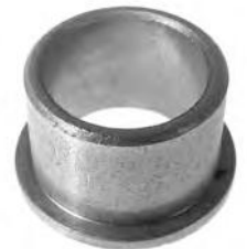
STC7102 Bushing, D/E For Tecumseh Starters PIC 6-15080; ID 12.7mm OD 15.93mm OAL 11.43mm 19.0mm Flange Used on Tecumseh Starters
